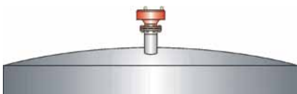
Figure 1: Free venting of the storage tank with PROTEGO® EH/0S
