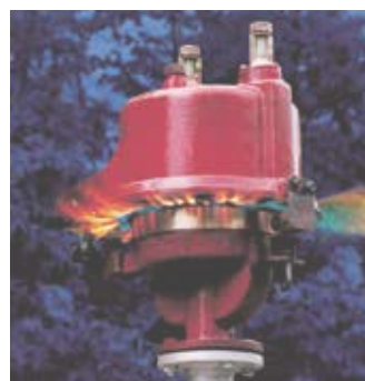
Figure 3a: Endurance-burning test with diaphragm valve PROTEGO® UB/SF
