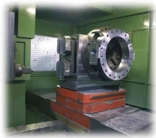
The welding process is totally automated, to obtain the best quality of chemical and mechanical characteristics. Stainless steels, duplex, stellite, Monel, Hastelloy, Inconel and all other alloyed materials are overlay welded on the seats maintaining their characteristics of resistance to corrosion and temperature with the highest hardness.
